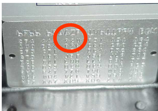
VIN PLATE FRONTERA PAINTCODE = 92U
